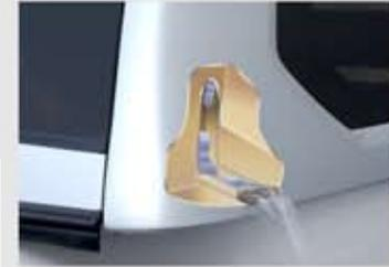
LATERAL DRAIN TO PREVENT WATER GETTING INSIDE THE VEHICLE.
