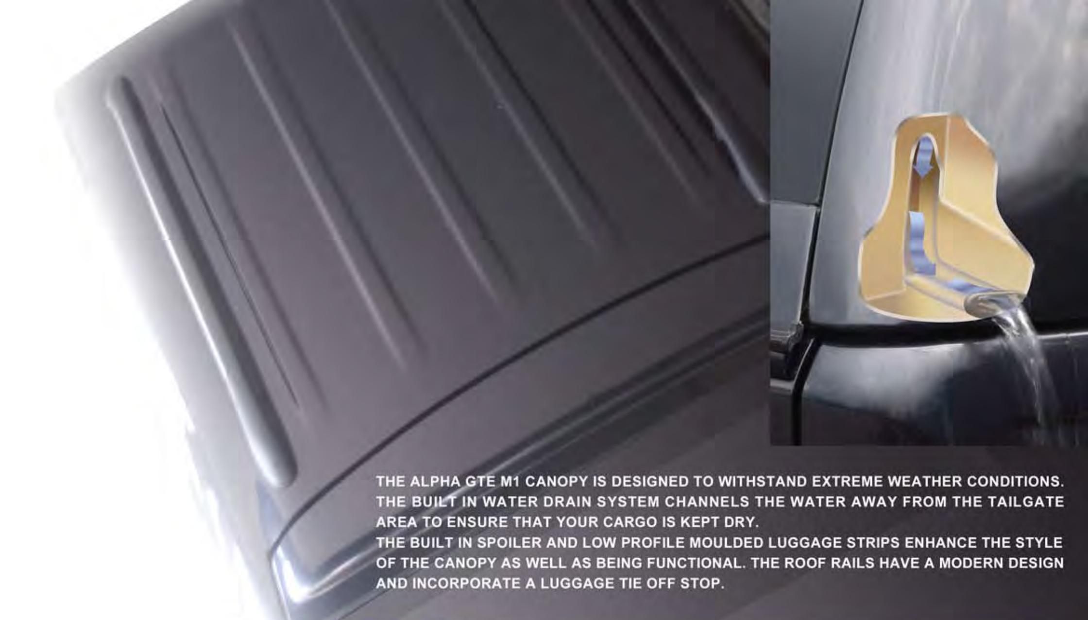
THE ALPHA GTE M1 CANOPY IS DESIGNED TO WITHSTAND EXTREME WEATHER CONDITIONS. THE BUILT IN WATER DRAIN SYSTEM CHANNELS THE WATER AWAY FROM THE TAILGATE AREA TO ENSURE THAT YOUR CARGO IS KEPT DRY. THE BUILT IN SPOILER AND LOW PROFILE MOULDED LUGGAGE STRIPS ENHANCE THE STYLE OF THE CANOPY AS WELL AS BEING FUNCTIONAL. THE ROOF RAILS HAVE A MODERN DESIGN AND INCORPORATE A LUGGAGE TIE OFF STOP.
