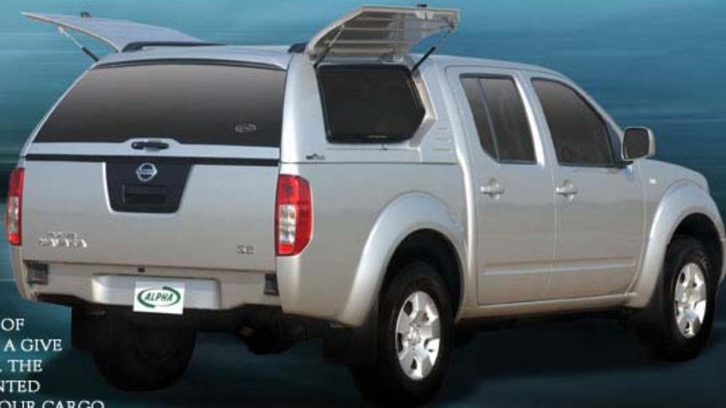
THE SOLID FIBERGLASS SIDE LIFT UP DOORS OF THE CML CANOPY ARE DOUBLE SKINNED TO GIVE A SMOOTHER FINISH AND EXTRA STRENGTH. THE REINFORCED SIDE DOORS KEEP OUT UNWANTED GUESTS BUT ALLOW YOU EASY ACCESS TO YOUR CARGO.
