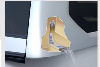
LATERAL DRAIN TO PREVENT WATER GETTING INSIDE THE VEHICLE.
