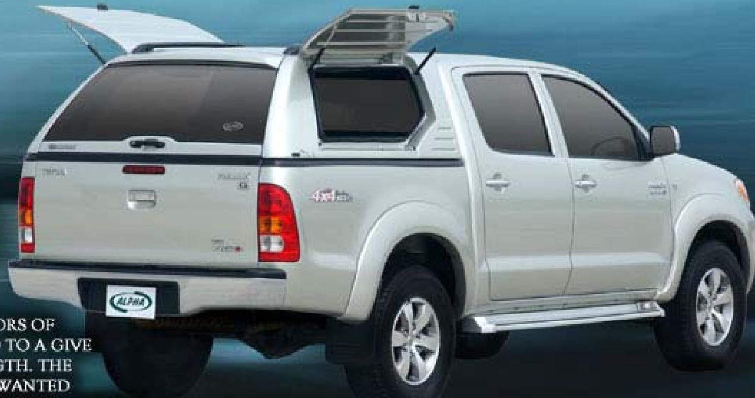
THE SOLID FIBERGLASS SIDE LIFT UP DOORS OF THE CML CANOPY ARE DOUBLE SKINNED TO A GIVE A SMOOTHER FINISH AND EXTRA STRENGTH. THE REINFORCED SIDE DOORS KEEP OUT UNWANTED GUESTS BUT ALLOW YOU EASY ACCESS TO YOUR CARGO.
