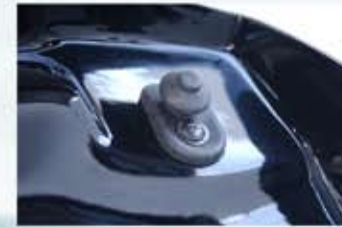
JAMB SWITCH. AUTOMATICALLY ACTIVATES THE INTERIOR LIGHT WHEN THE REAR DOOR IS OPENED.
